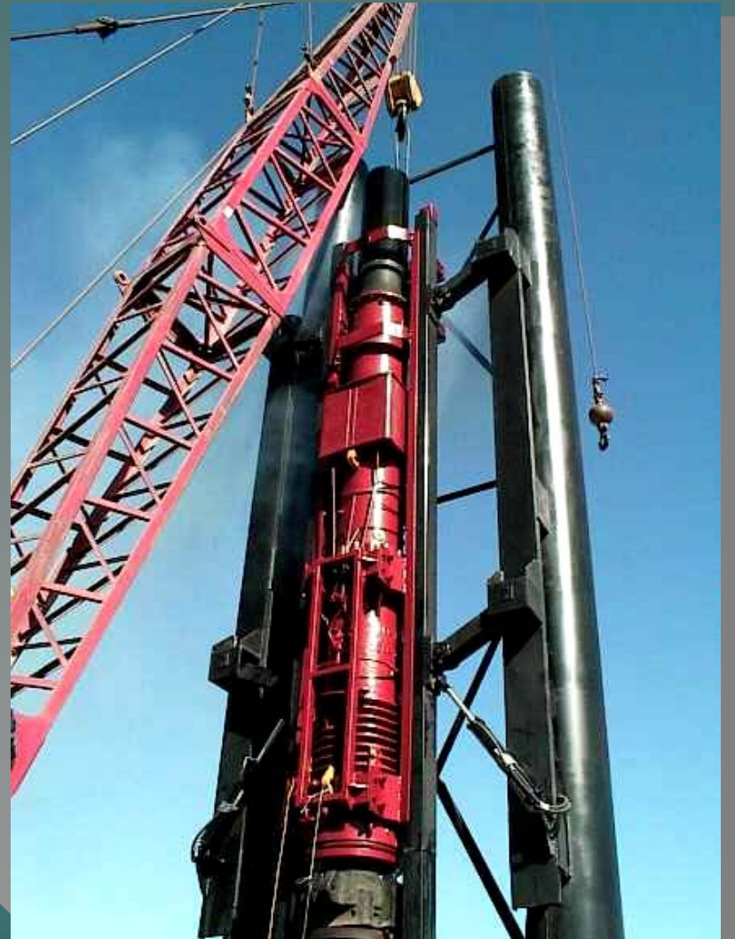
APE D-46-32 at full stroke on test stand in California undergoing sound tests.
